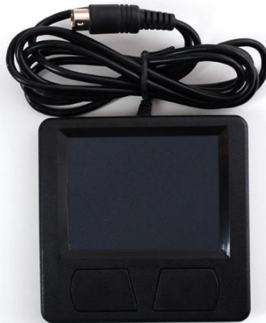
Figure 3.6.2 of Capacitive Trackpad/Touchpad
